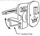
If necessary, move the support leg to the alternate bracket holes.
